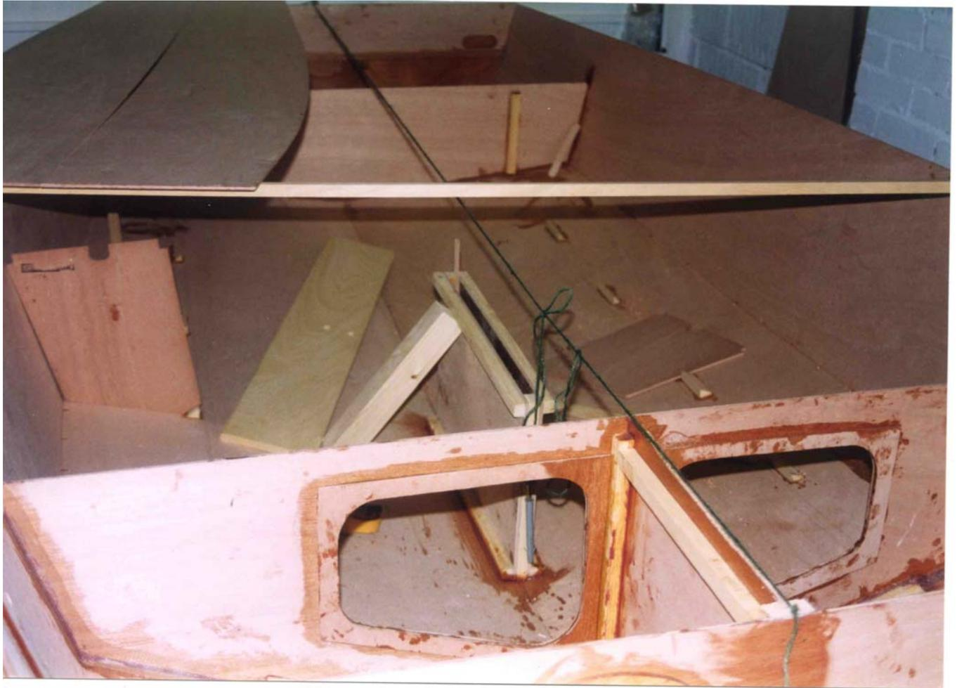
**This photo shows the rear deck support glued into place and the seams taped prior to fixing the rear deck. The tank is also coated in epoxy.**
