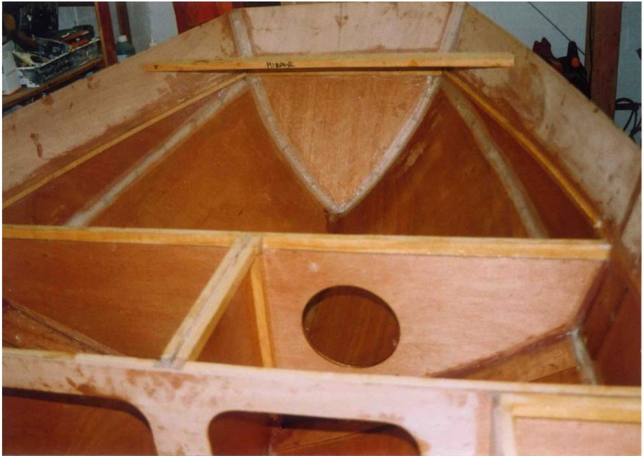
**The side tanks just prior to deck Fixing. Note that the bulkhead needs to be fixed directly in line with the thwart.**
