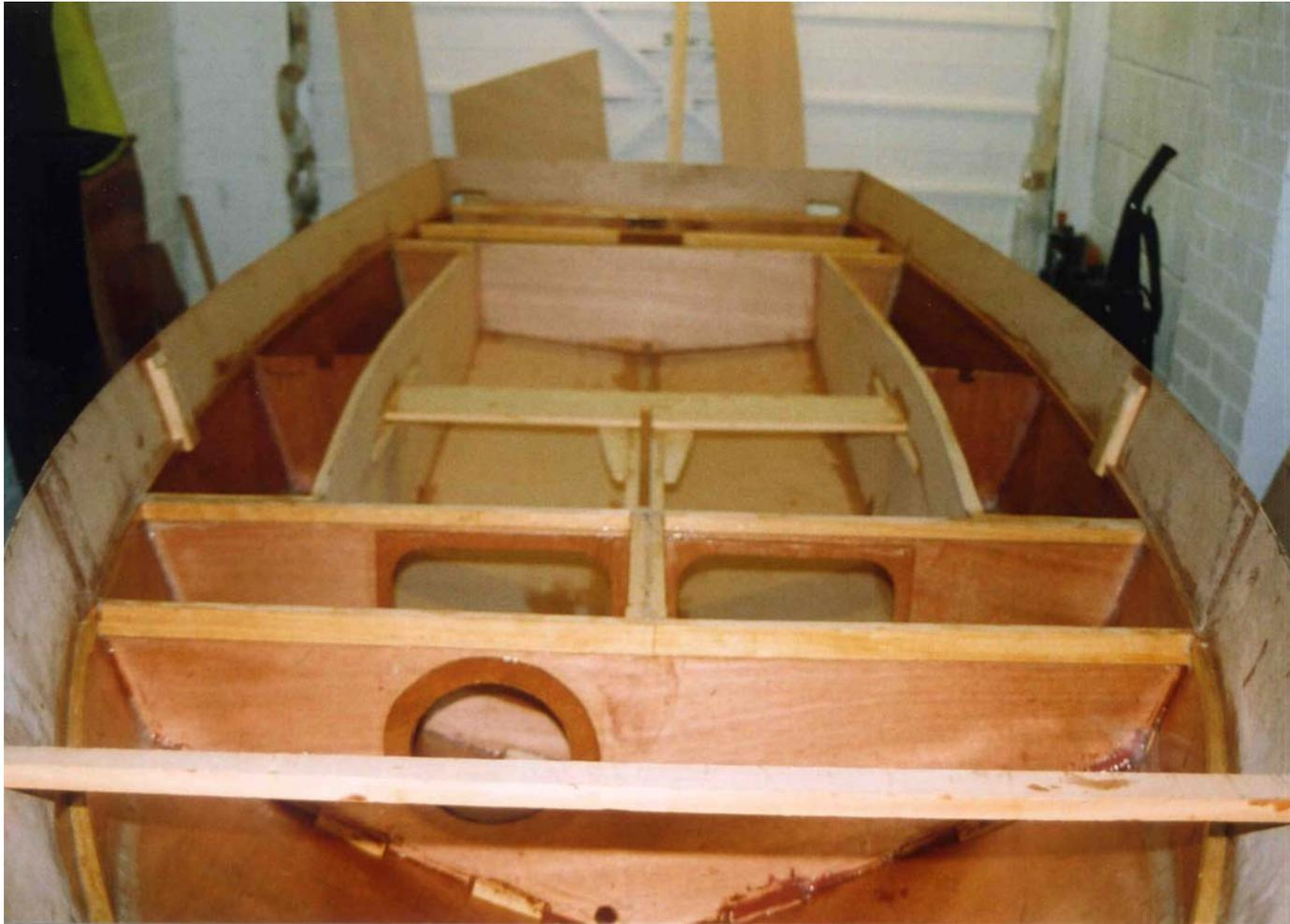
**The final step is fixing the decks to the hull. By this stage all the internal structure is complete and the tanks coated in epoxy. The fitting of the decks suddenly makes the kit look like a boat.**
