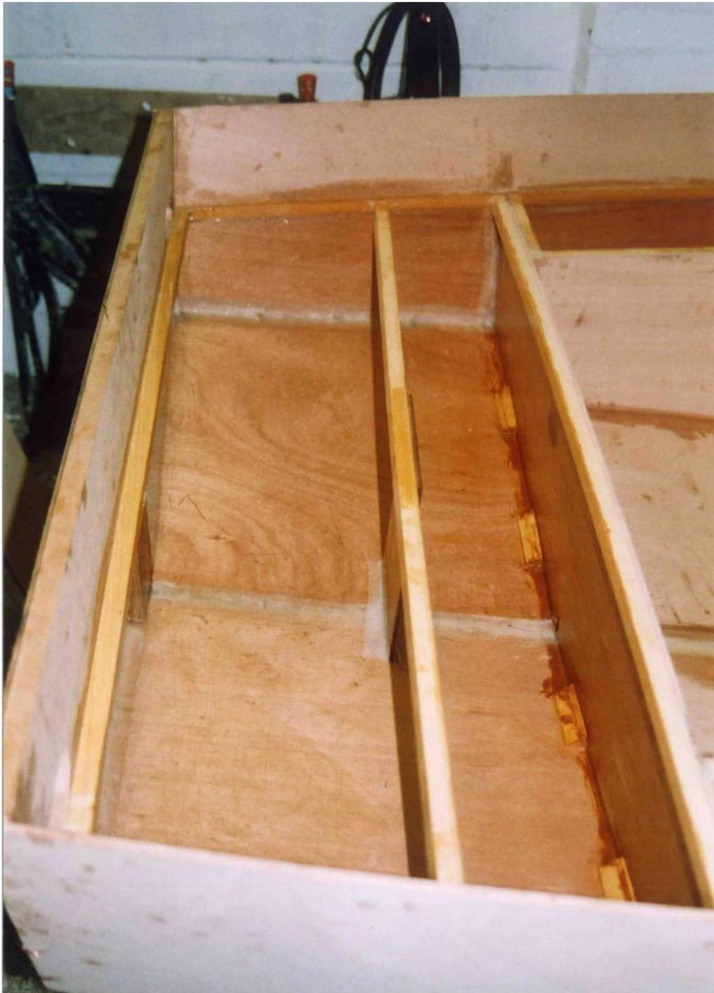
**This photo shows the forward tank and bulkhead prior to fixing the fore deck. The battens that support the deck are in place and all the taped seams.**
