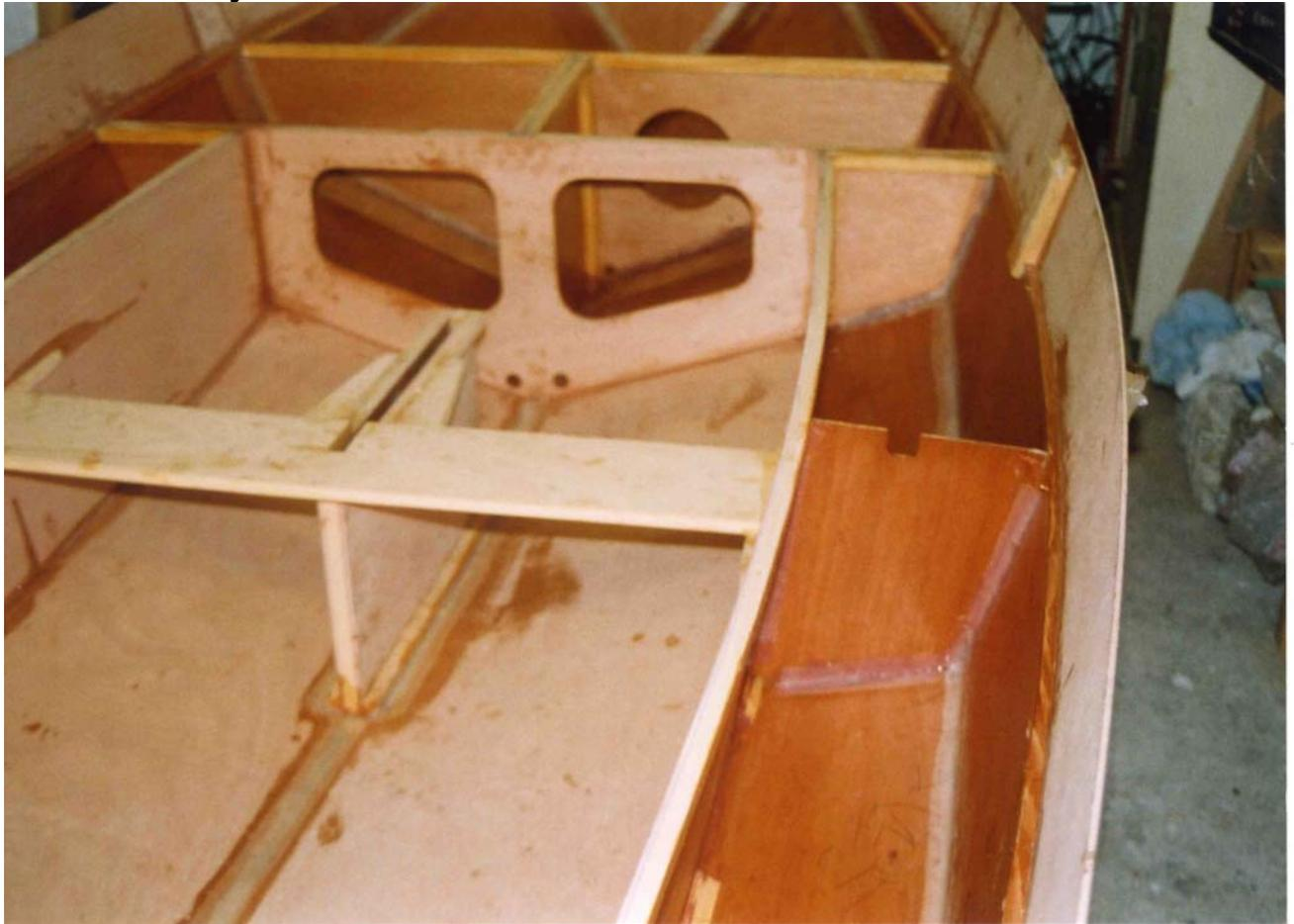
**This Pictures shows the boat prior to fitting the decks. By this stage all the bulk heads and thwart had been glued in and all the seams taped. The temporary strut at the front held the bow in shape prior to fixing the decks. You will see that all the tanks have been coated in West. 3 coats were used as there is no 2nd Chance!**
