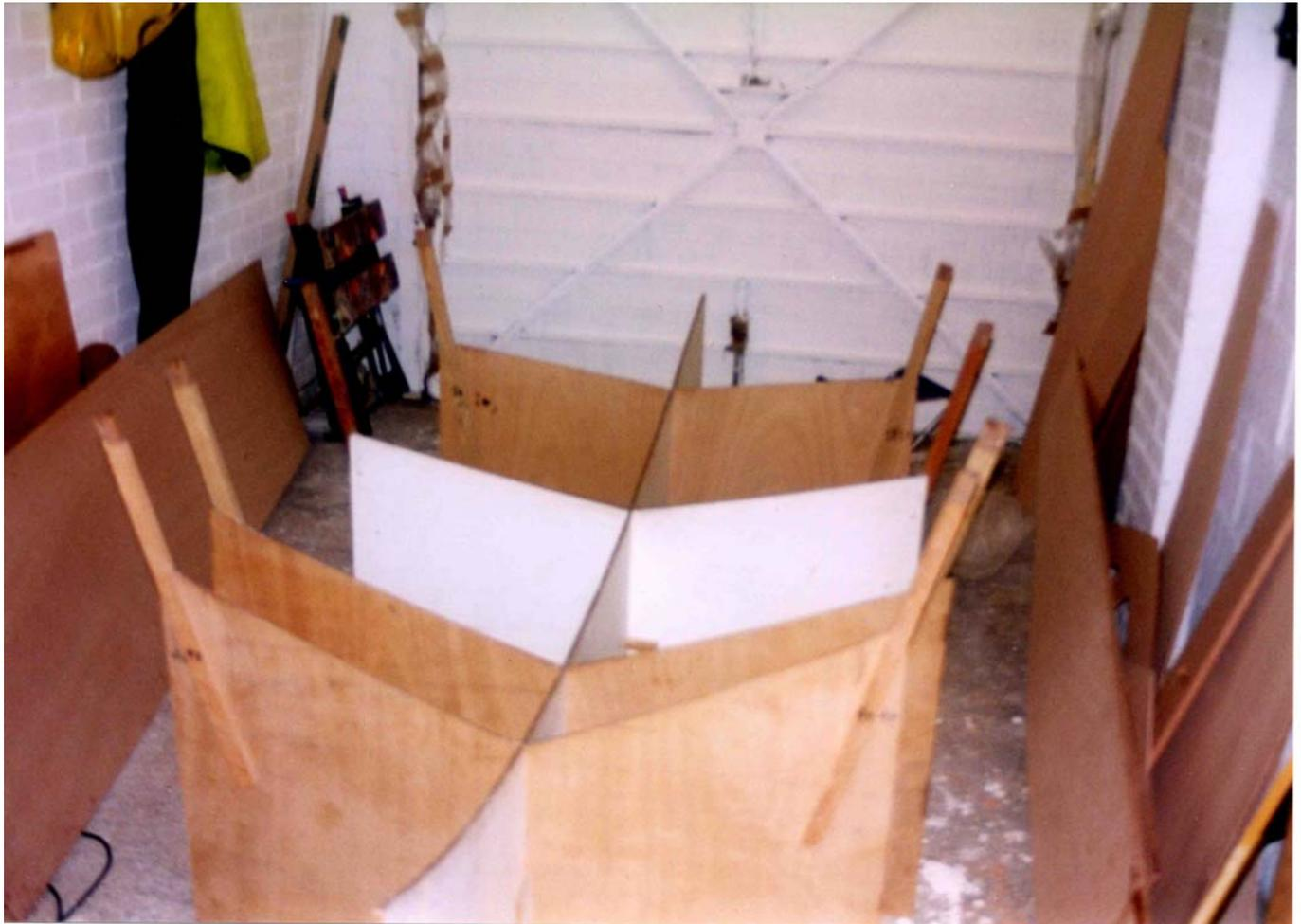
The Main Panels were fixed to the Jig, requiring minor reshaping of the supplied panels to make best use of the tolerances within the Mirror class rules. All the top boats now follow a similar principle of flat aft sections and maximum curvature, and hence buoyancy, towards the front. It is practical to make the jig to match an existing boat's measurements.
